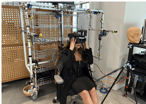
Figure 2. Stationary configuration for inclusive capture. The rig can be mounted statically to allow for seated data collection. This setup eliminates the weight burden of the backpack, accommodating participants with limited mobility or physical endurance.
