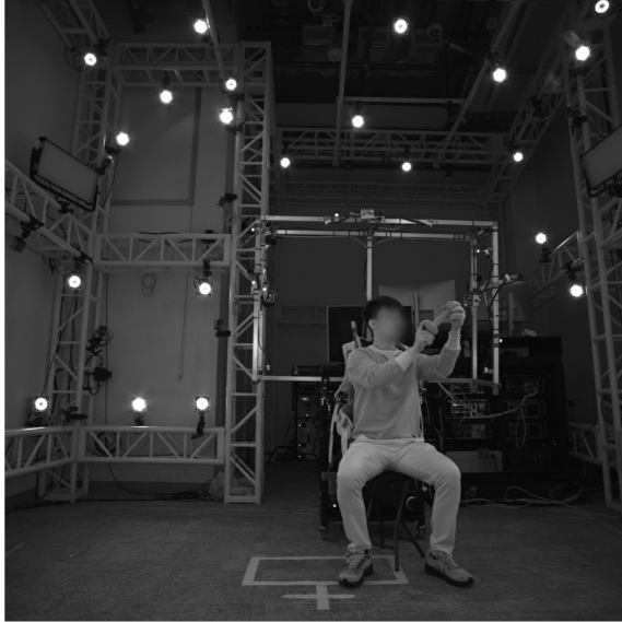
Figure 5. Simultaneous rig-dome capture for ground truth validation. To evaluate the accuracy of our mobile annotation pipeline, we captured sequences where the subject wears our mobile rig inside a high-fidelity stationary multi-camera dome. This allows for a direct comparison between our mobile-rig-derived annotations and the dome-derived “gold standard.”
