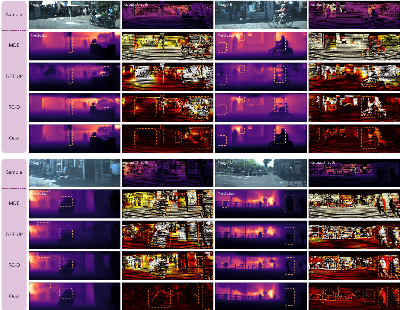
Figure 2. Additional qualitative comparison on VoD. POLAR more accurately predicts metric scale, and exhibits fewer global misalignments and geometric artifacts in comparison to other methods. Polynomial fitting, allowing POLAR to non-uniformly scale distinct local regions, results in notable improvements in metric depth estimation over initial MDE predictions. This is apparent in all MDE error maps: though object depth geometry is reasonable, actual metric depth values tend to be inaccurate. GET-UP, while marginally improving metric depth estimation relative to MDE, presents substantial errors in depth structure. For instance, the presence of geometric artifacts or omission of objects or regions entirely can be seen through the following highlighted examples: loss of motorcycle body and visor in Image A, front portion of biker (right) and bike wheel (far-left) in Image B, top of motorcyclist in Image C, and street sign in Image D. RadarCam-Depth (RC-D) similarly exhibits geometric artifacts, present in the sign pole, motorcycle, and fence post in Image A, biker and bicycle wheel in Image B, roof overhang and motorcyclist in Image C, and fence posts and pedestrians in Image D. In contrast, POLAR extrapolates correct structure from photometric priors while also demonstrating clear improvements in metric depth fidelity compared to all other baselines.
